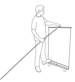
4. Insert the pole onto the cup of the base.
